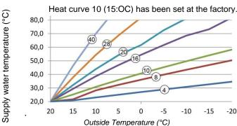
Heating curve ratio is at room temperature setting of 20 °C
