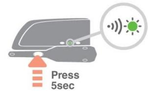
2. **LED turns OFF on Gateway and Gateway icon disappear on Round, indicating that binding has been cleared.**
