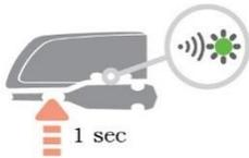
Put Round into BIND mode by pressing the right touch-button under the display for 10 seconds.
