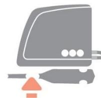
LED on Gateway should turn solid green when successfully registered.
