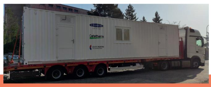
Cetetherm s.r.o. in Czech Republic supplied an 8 m length cooling substation of 15 tons fitted in a specific designed container for delivery to Oulu, a Finnish town close to the Polar circle. Cetetherm cooling technology will be part of a formic acid production on site.
